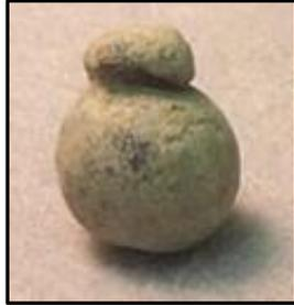
By the time of the Civil War, most U.S. balls were being "swaged"; the cold lead being formed by two dies coming together to literally stamp out a round ball with NO sprue mark.
